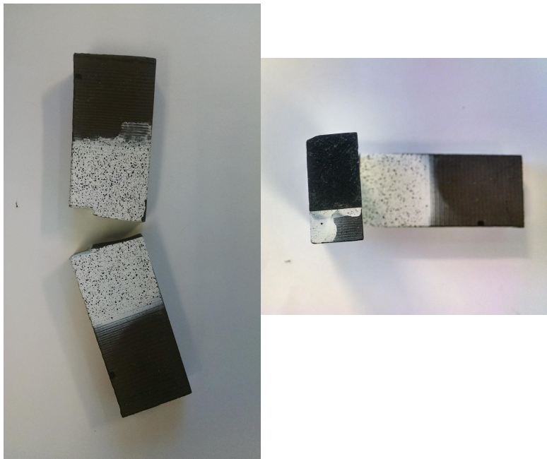
Figure 17: Marcellus shale specimens after failure in three point bending tests.
