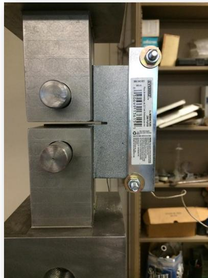
Figure 3: a) Experimental setup considered in the analysis, and b) new massive grips designed to achieve stable postpeak
