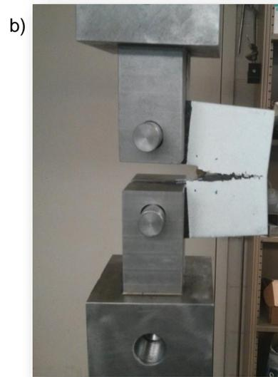
Figure 8: a) Example of MTS standard grip and b) newly designed grips of increased stiffness and mass
