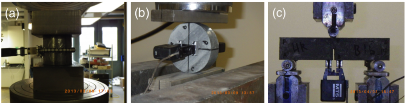
Figure 2: UHPC experiment setup: (a) cylinder compression, (b) splitting, (c) beam 3-point-bending
